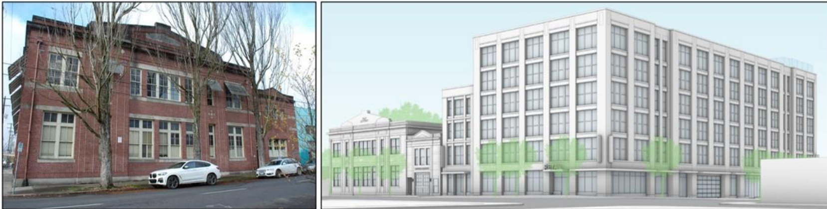
This massing study illustrates a new addition on right that is larger than the historic building (Troy Laundry building in Portland). The new building employs a “sidecar” to transition the mass of the new building addition and relate it to the older building. (Source for image on right: Hartshorne Plunkard Architecture)
